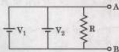
where value of  $V_2 = 5 \text{ V}$ . The internal resistances of both the batteries are  $0.1 \Omega$ . The current through the resistance  $R$  is about:
